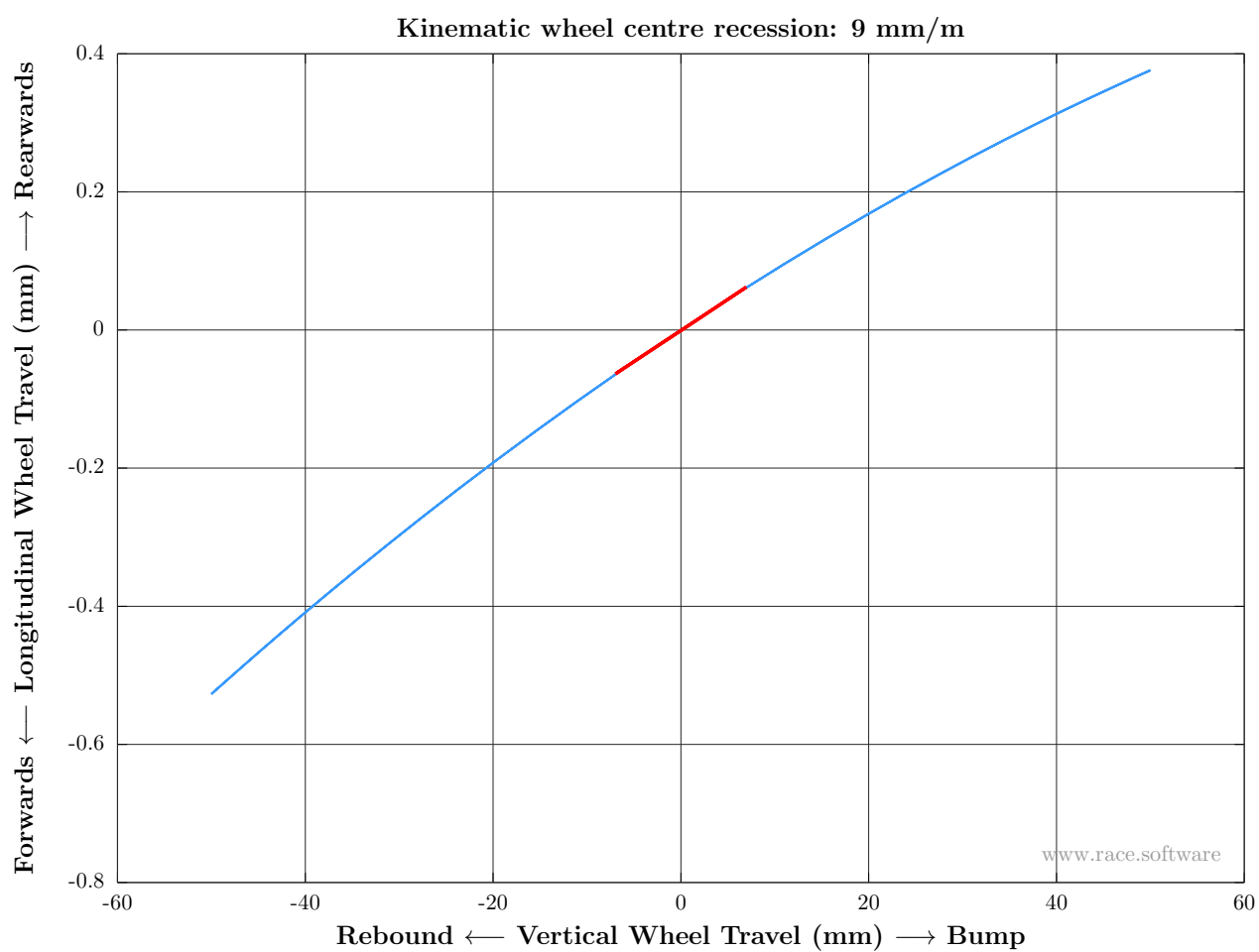
Figure 12: Vertical test: Kinematic wheel centre recession
