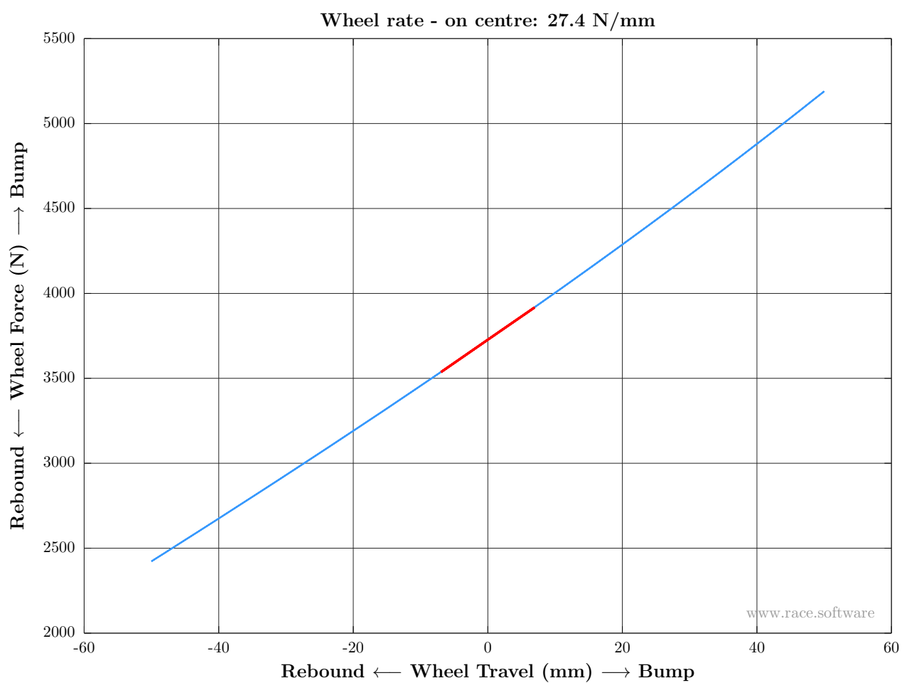
Figure 14: Vertical test: Wheel rate - on centre
