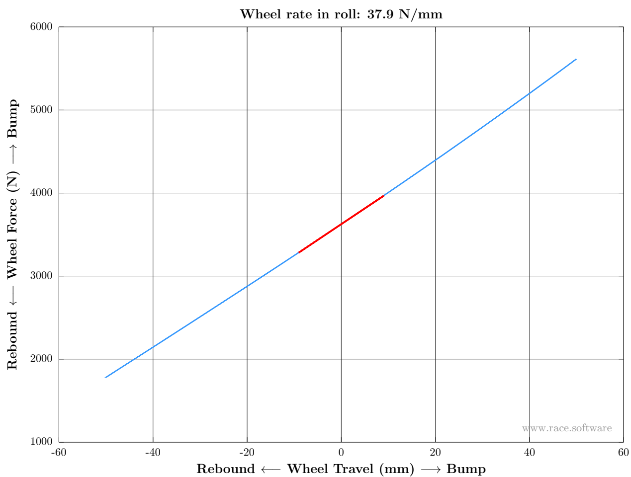
Figure 34: Roll test: Wheel rate in roll
