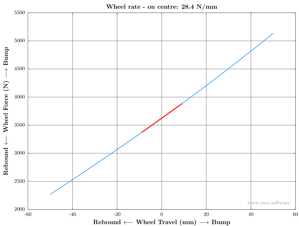
Figure 26: Vertical test: Wheel rate - on centre
