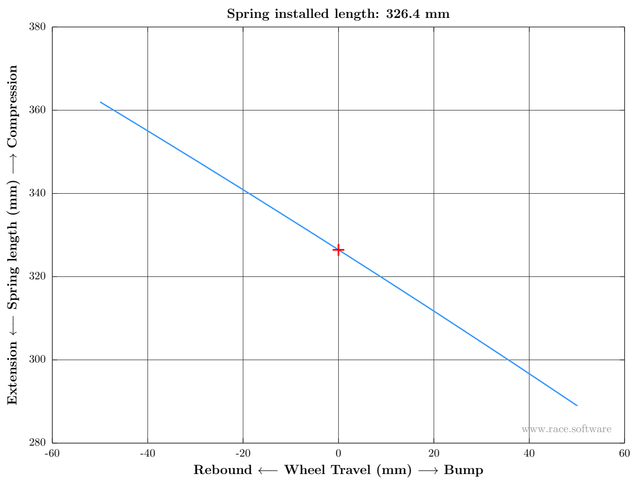
Figure 18: Vertical test: Spring installed length
