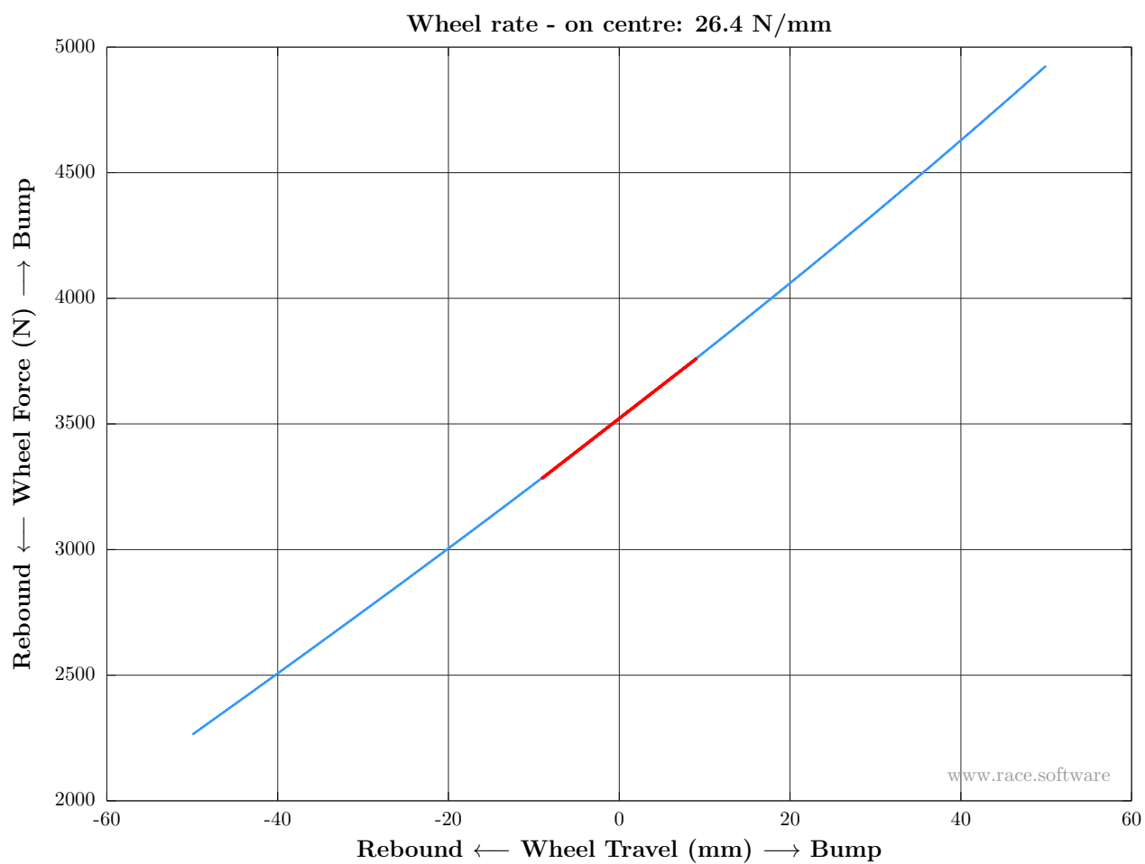
Figure 14: Vertical test: Wheel rate - on centre
