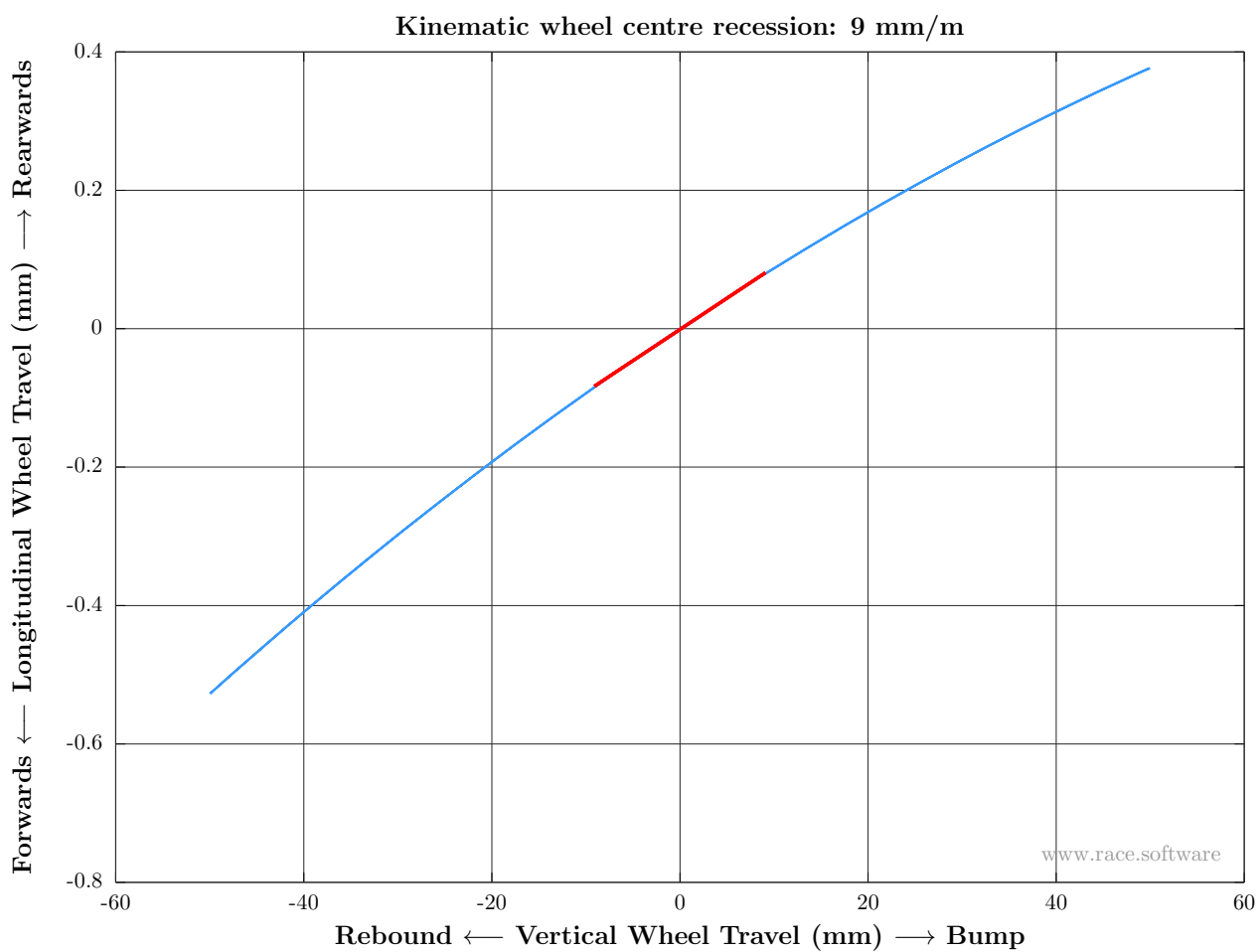
Figure 12: Vertical test: Kinematic wheel centre recession
