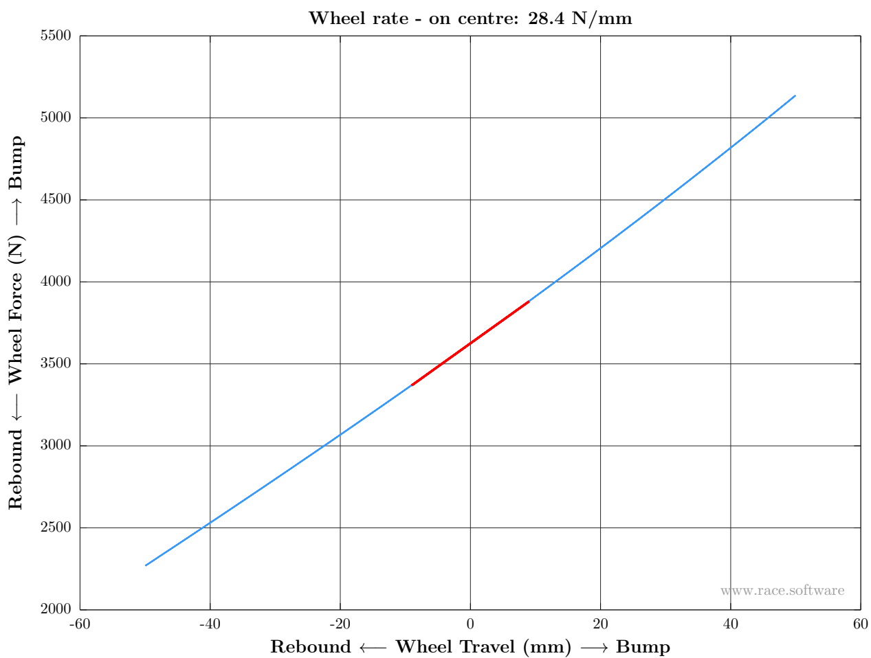
Figure 26: Vertical test: Wheel rate - on centre
