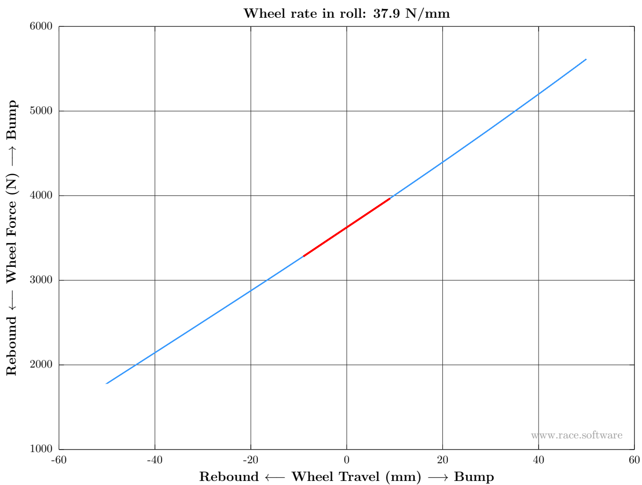
Figure 34: Roll test: Wheel rate in roll
