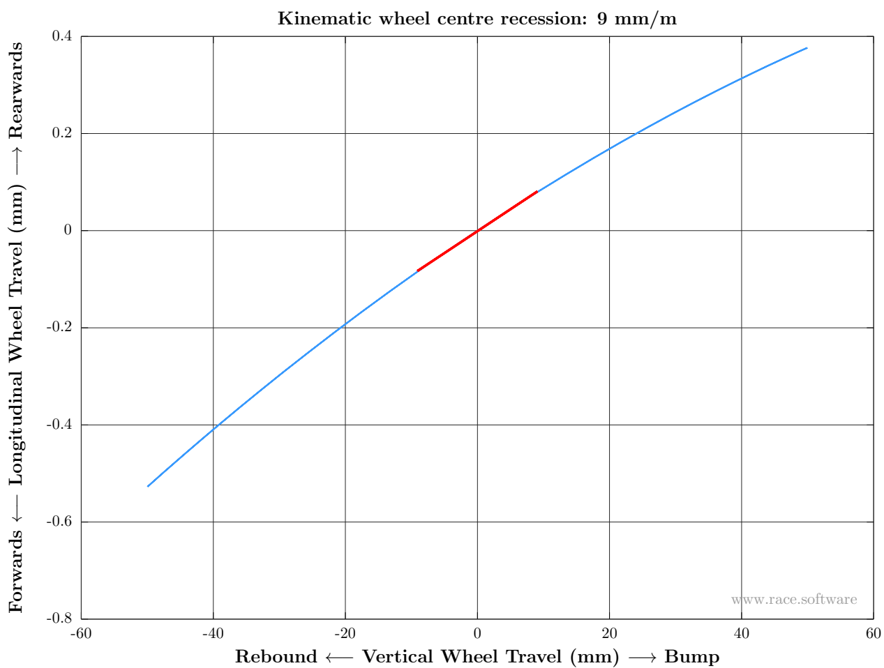
Figure 12: Vertical test: Kinematic wheel centre recession
