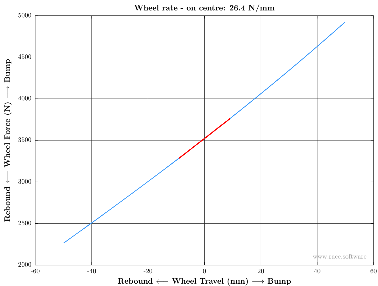
Figure 14: Vertical test: Wheel rate - on centre
