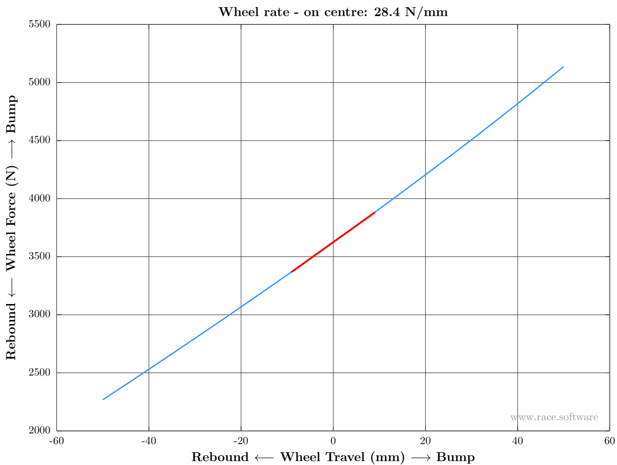
Figure 26: Vertical test: Wheel rate - on centre
